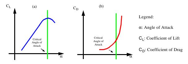
Figure 5. Graph of Angle of Attack vs. Coefficient of Lift and Coefficient of Drag[3]
