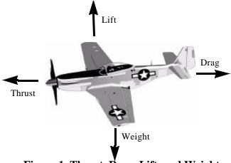
Figure 1. Thrust, Drag, Lift, and Weight
