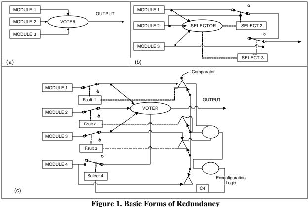
(a) Fault Masking with TMR; (b) Reconfiguration; (c) Hybrid TMR
