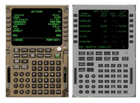
Figure 9. CDU panels from Boeing 747 (left) [14] and MD-11 (right) simulations
