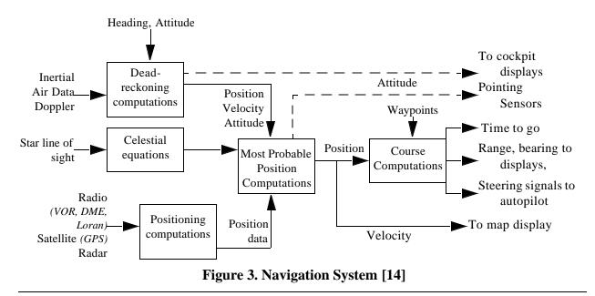
instantaneous and continuous; they are self-contained, making them un-jammable; measurements can be made independent of weather or geographical location; and they are able to produce position and ground-speed information[14].
