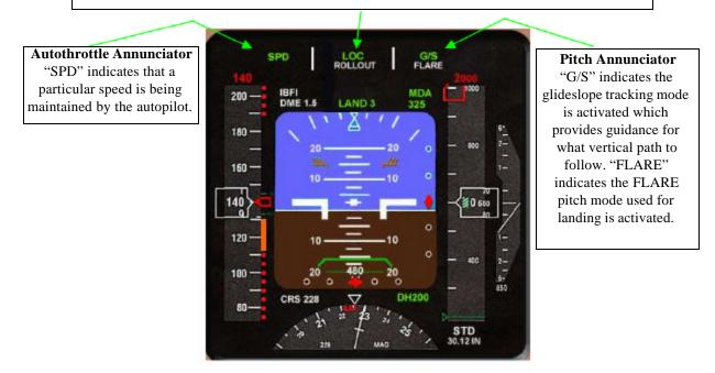
Figure 2. MD-11 (top) and B-747 [14] (bottom) Primary Flight Displays
