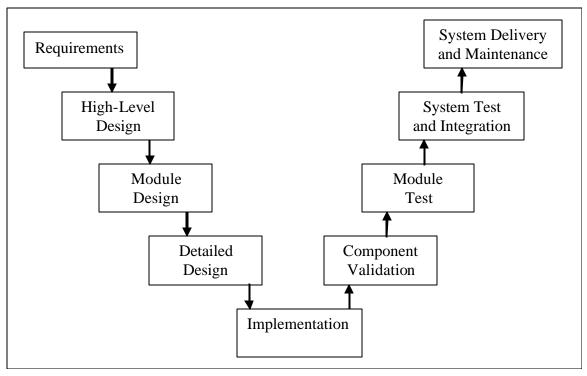
Figure 3. A Typical Software Lifecycle
