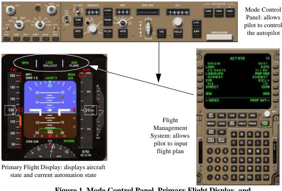
Figure 1. Mode Control Panel, Primary Flight Display, and Flight Management System relationship (images from [14])
