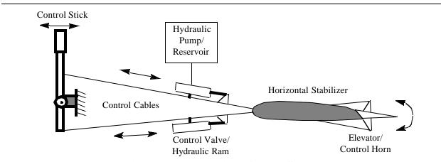
Figure 2. Boosted Flight Control System
