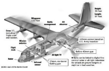
Figure 2. Illustration of the AC-130.
