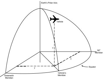
Figure 1. *x*, *y*, *z* Coordinate Frame[13]
