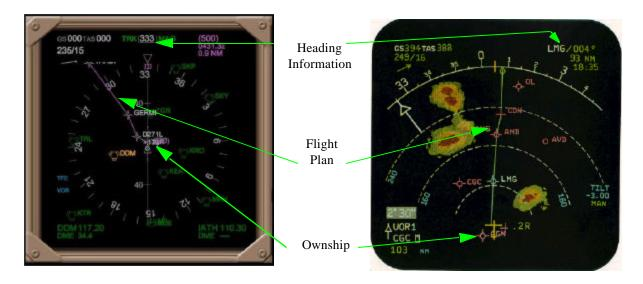
Figure 6. Boeing 777 ND [14] (left) and A320 ND [5] (right)
