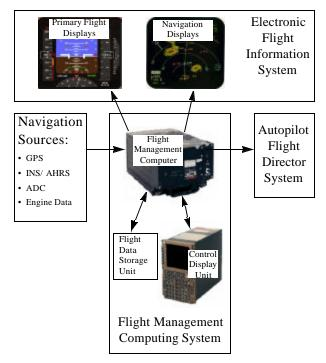
Figure 7. FMS Components
