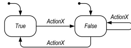
Fig. 4. Finite state transition description for *CX* where *X* can be 1, 2, 3 or 4. *CX* can start out being either true or false. If *CX* is true and the human operator performs *ActionX*, *CX* becomes false. If *CX* is false and the human operator performs *ActionX*, then *CX* can either become true or remain false.
