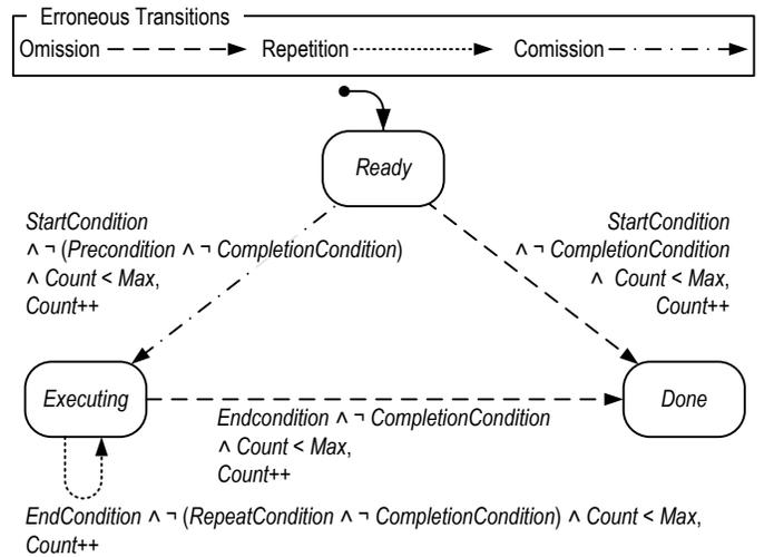
Fig. 2. Additional EOFM activity formal semantic transitions for generating erroneous behavior beyond the normative transitions shown in Fig. 1(a).
