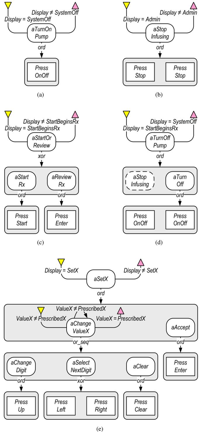
Fig. 8. Visualization of the instantiated EOFM for normatively programming prescriptions into the PCA pump. Note that (e) represents a generic pattern for programming value  $X$  into the pump where  $X$  can be *PCADose*, *Delay*, or *Limit*. Also note that the dotted line around *aStopInfusing* in (d) indicates that *aTurnOffPump* is referencing the activity *aStopInfusing* defined in (b).
